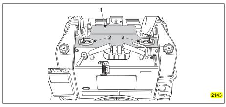
Figure 4-6 Remove Upper Inspection Panel
